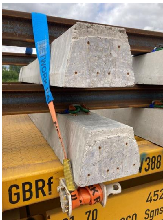
Diagram 2: Acceptable option where the securing strap is positioned between the sleepers and deviates around the sleepers due to the wagon winch position being obstructed.
