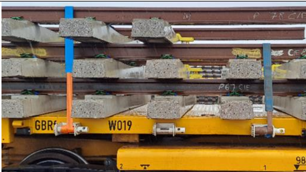
Diagram 1: Preferred option where securing straps are positioned between the sleepers without any deviation of the securing strap.
